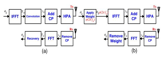
Fig. \2. Simplified block diagrams for an OFDM system with (a) convolution scheme and (b) proposed weighting scheme.
