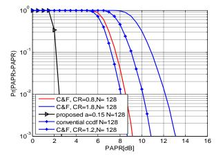
Fig: 4 Comparative PAPR reduction in MIMO OFDM Systems CCDF of the C&F and proposed methods for N = 128
