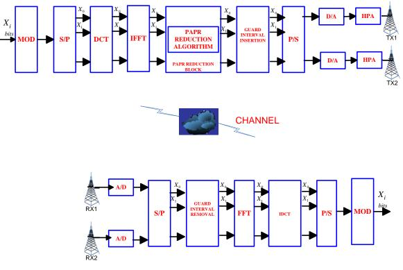
Fig.1. PAPR reduction system model in MIMO-OFDM SYSTEMS
