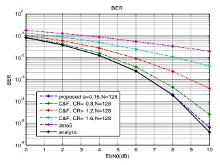
Fig: 3 Performance analysis of PAPR reduction in MIMO OFDM Systems BER of the C&F and proposed methods for N = 128
